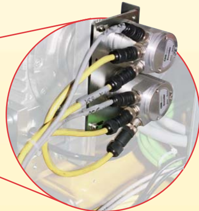
Example of an application where two Pluto Safety Encoders provide safe position determination in a gantry robot.
